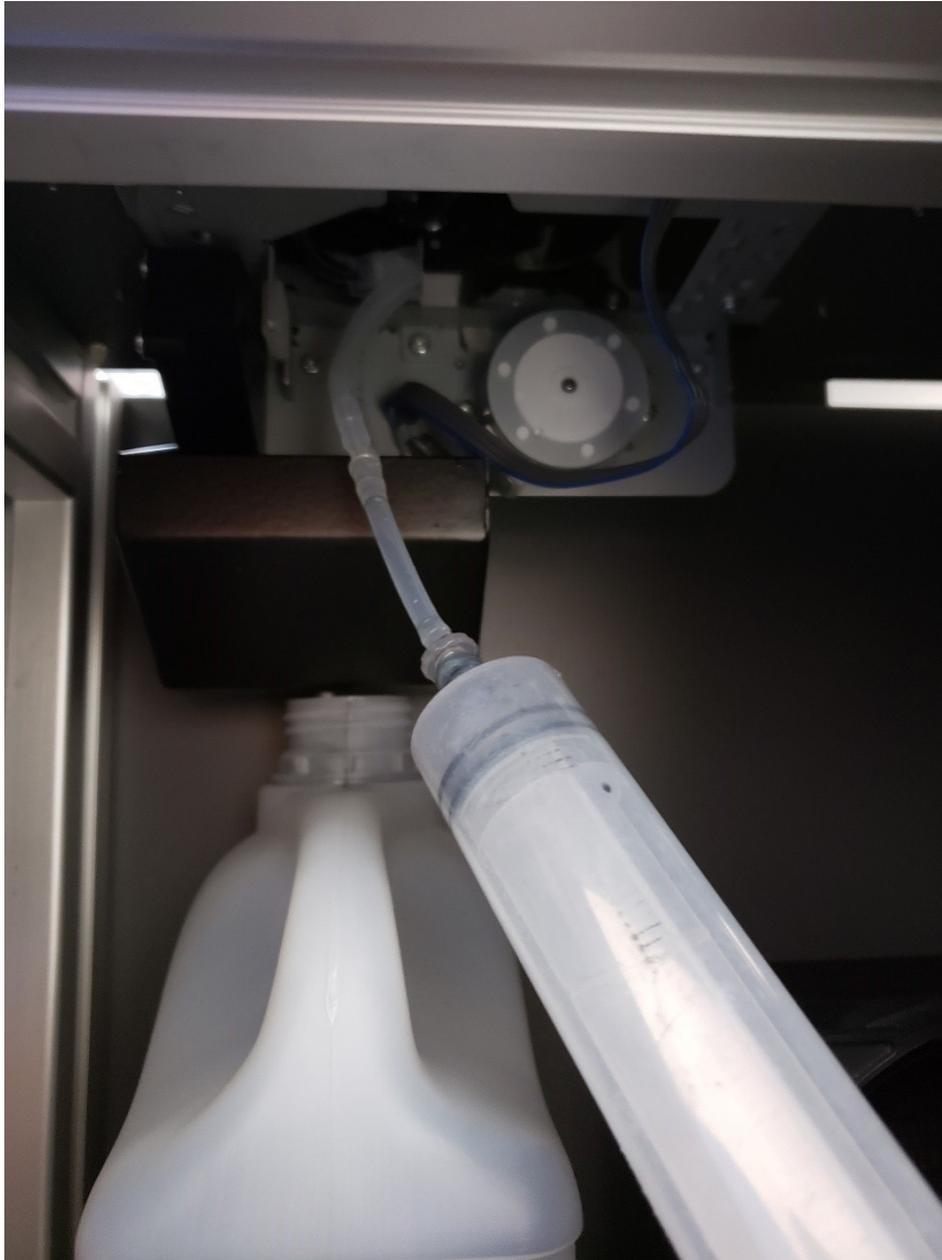
If the syringe test indicates the capping station is functioning normally, proceed with more aggressive cleaning procedures.
